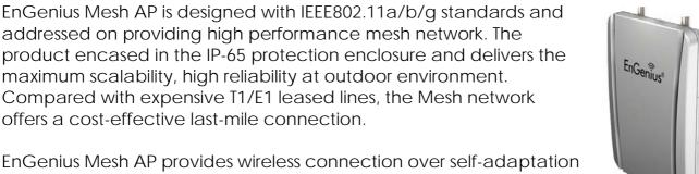
offers a cost-effective last-mile connection. EnGenius Mesh AP provides wireless connection over self-adaptation mesh backhaul (5GHz). The mesh AP can operate at 2.4GHz for long range interference. The detachable antenna design allows users to
